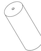
*Tip: If enlarging an existing hole, try cutting a dowel of the appropriate size to use as a guide for the hole saw.*
