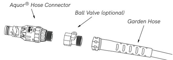
**!** *Some Aquor® hose connectors have a one-way check valve to prevent water from spraying when you disconnect.*
